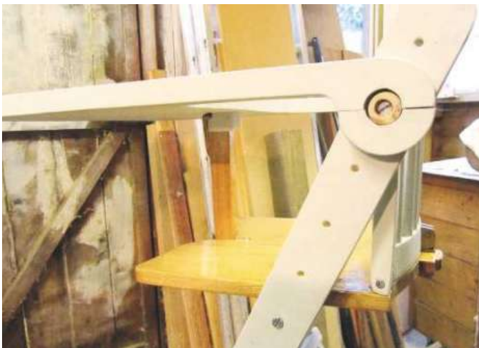
▲ Pic.10 A flat-bladed screwdriver and a few minutes is all that's needed to undo the bolt and screw on each side and move the seat to a different pair of holes
